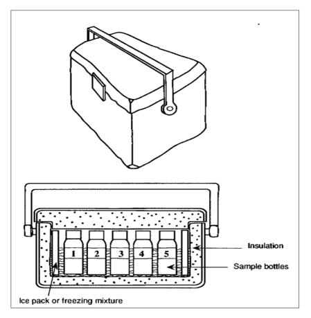
Figure 8.6: Insulated bottle carrier for water quality samples
