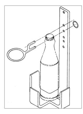
Figure 8.1: Sample bottle holder for water sampling
