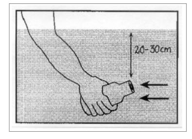
*Figure 7.2: Collecting a sample from surfce water*
